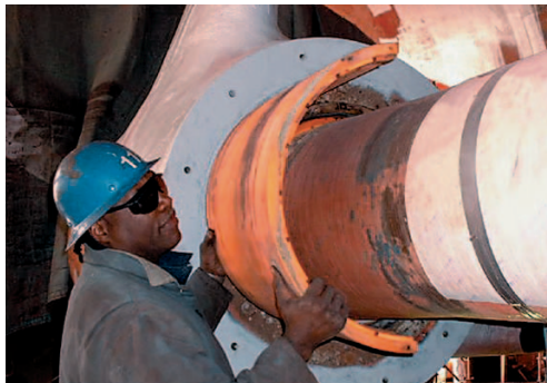
COMPAC with tapered key design allows the bearing to be withdrawn, inspected and re-installed or replaced in a few hours.
